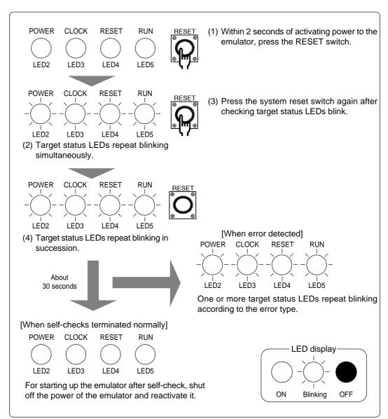
Figure 5.2 Self-check procedure
